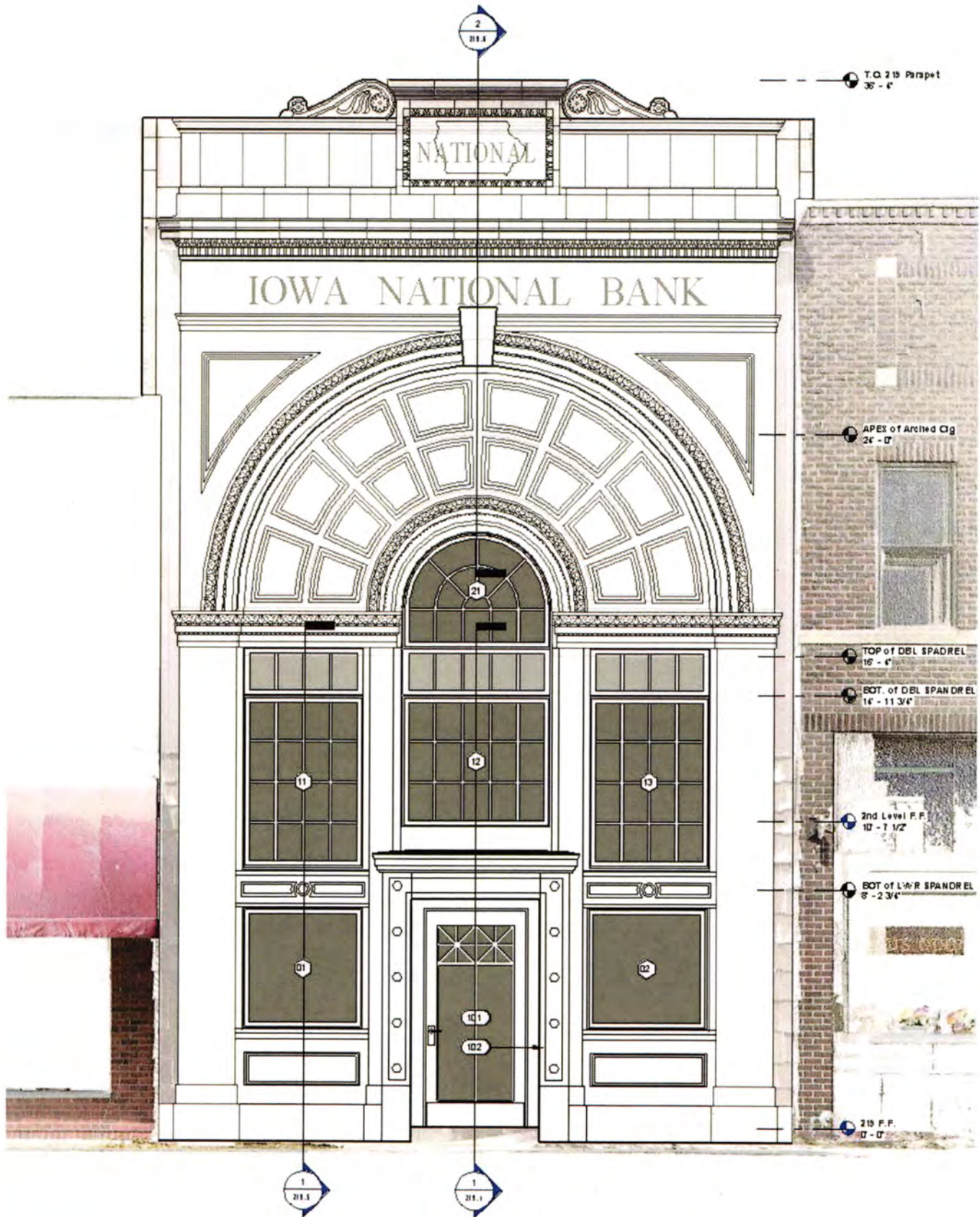
1 Southwest Facade 219 - NEW CONSTRUCTION 3/8" = 1'-0"
