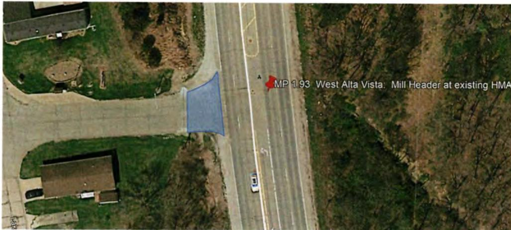
Iowa 149 general concept mill 2" 1" HMA Interlayer, plus 1.5" thick HMA. Net increase +0.5" higher profile. (north of RR bridges an additional 1.5" HMA NB and 1.5" SB north of Angle Rd)
